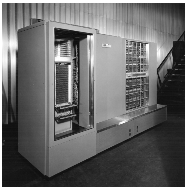
Figure 3. (a) A general view of an IBM 704 computer of the type at Argonne National Laboratory used by members of LMSS. At the center of the figure is the operators console, to the left is a card reader used to input programs and data; just to the right of the card reader is an impact printer. At the far left is a portion of the CPU where some of the vacuum tube logical units are shown. (b) A close-up of the CPU showing, on the right, in more detail the vacuum tube logical units. (Courtesy of IBM Archives.)
