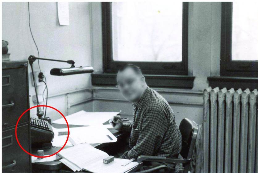
Figure 4. A Mathematical Assistant at LMSS, using an electric calculator to check results obtained with computer programs. (Courtesy of Hidemi Suzuki.)
